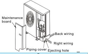
The cable wire can be led from the back hole of the pipinghole or ejectinghole.
