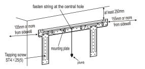
NOTICE: The holes at solid arrow position must be secured to avoid the shake of mounting plate.
